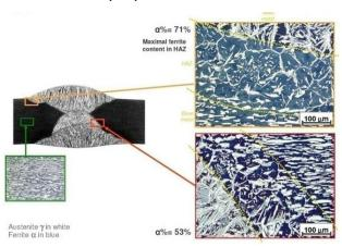
**2.4. To prevent phase precipitations** which will reduce corrosion as well as mechanical properties (ASTM A923)
